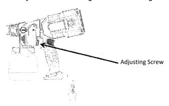
9. Spray pattern adjustment. Turn the knob to adjust from round pattern to fan pattern.
